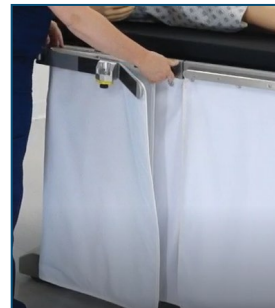
Slide Wing Shield onto table rail and secure with tightening knob. As shown below, pull corner plunger to release wing part of shield
