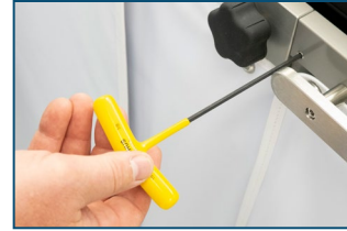
Use Allen wrench to tighten (or loosen) set screws at both ends of the shield to secure to rail
